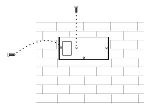
3.Connect the cable to the socket of the indoor monitor, then hang it on the bracket.
